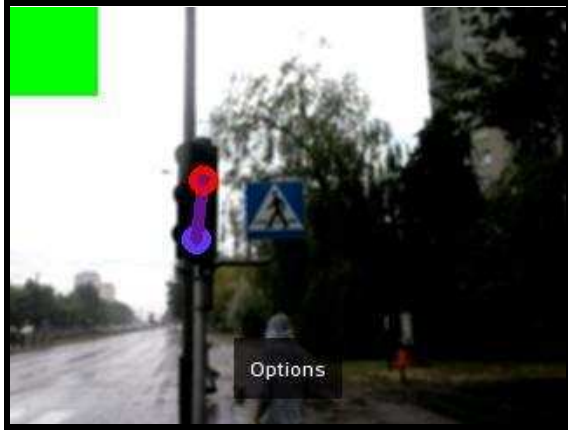
Figure 6. Screenshot from smartphone display while the application detects traffic lights change
